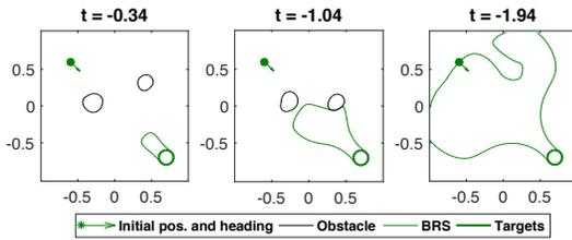
Fig. 2: Evolution of the BRS and the obstacles induced by  $Q_1$  and  $Q_2$  for  $Q_3$  in the centralized control method.
