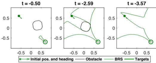
Fig. 4: Evolution of the BRS for  $Q_3$  in the robust trajectory tracking method. Note that a smaller target set is used to ensure target reaching for any allowed tracking error.
