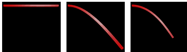
Figure 2: The left image shows a beam at its initial configuration with a fixed left end and a free right end. The middle image shows the distorted deformation under gravity, using linear strain. The right image shows the undistorted deformation, under the same gravitational force, using quadratic strain (equation (5) and (6)).
