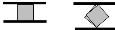
Figure 7: The grasp configuration on the left is stable; those on the right are not.
