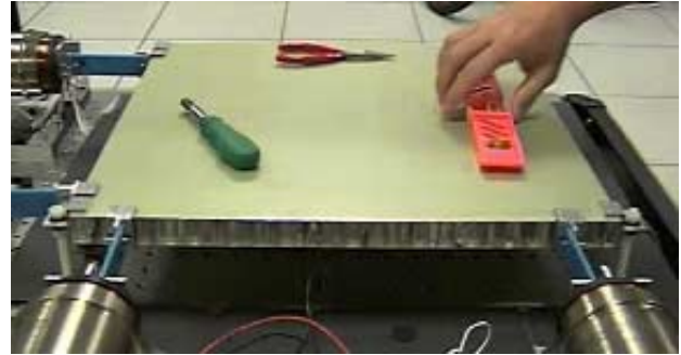
Figure 1: The Universal Planar Manipulator (UPM): generic objects placed on a flat plate can be manipulated independently via vibrations/friction.
