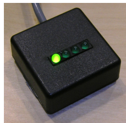
Figure 5. An LED next to each microphone lights up when the system is processing an audio command to let users know the system “heard” them.
