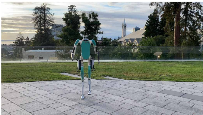
Movie 1. Outdoor deployment. A reinforcement learning-based controller enables real-world humanoid locomotion.
