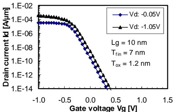
Figure 13: Simulation data for FinFET with 10-nm gate length.  $I_{\text{dsat}} = 347$  (or  $694$ )  $\mu\text{A}/\mu\text{m}$  for  $V_g = V_d = 1.2 \text{ V}$ , and  $I_{\text{off}} = 2.3$  (or  $4.6$ ) nA/ $\mu\text{m}$ .
