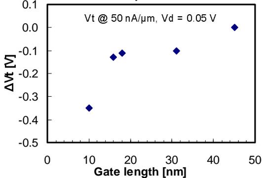
Figure 7:  $V_t$  roll-off characteristics
