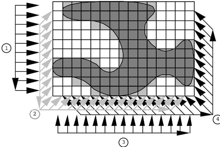
The scanner consists of four arrays of sensors arranged around a 10x15 matrix. Array 1 consists of 10 sensors pointing to the right, array 2 has 24 sensors pointing diagonally to the top right, array 3 has 15 sensors pointing to the top and array 4 has 24 sensors pointing to the top left. Each sensor records the thickness of that portion of the object directly in front of that sensor.
