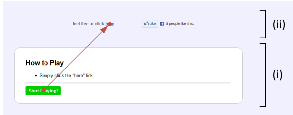
Figure 2: Workflow for our pointer destabilization attack. At first, (i) displays the instructions, and (ii) is hidden. When the player clicks the green button in the lower left, (i) disappears and (ii) appears. This ensures that the cursor approaches from a controlled direction (superimposed as the red arrow).
