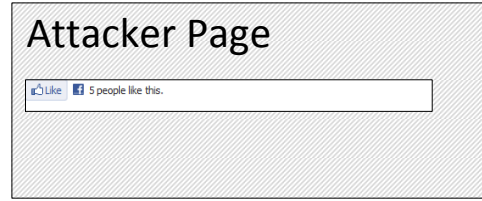
Figure 1: Illustration of our threat model. The attacker controlled page frames a page with a sensitive action, in this case, a Facebook Like button. The attacker has full control over the page (marked with grey background) except for the Facebook Like button frame (clear background), which must be fully visible for at least a second.
