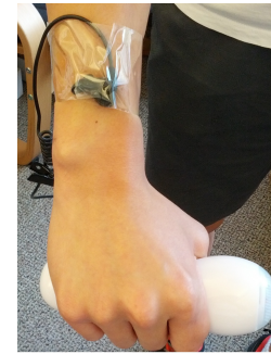
Figure 5: The setup and placement of our bone conduction microphone on a researcher’s wrist and the hand-held vibrator we used to transmit the intent signal.
