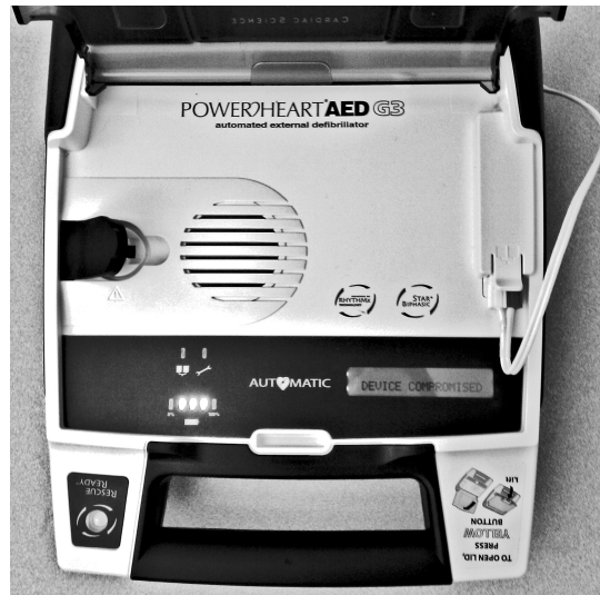
Fig. 1. The Cardiac Science G3 Plus exploited to install our custom firmware. The AED displays DEVICE COMPROMISED.
