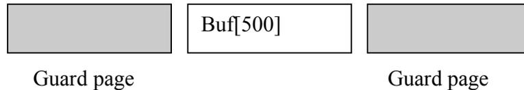
Electric fence uses an instrumented implementation of malloc.
