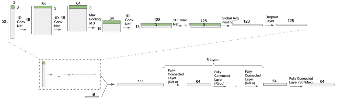
Fig. 2. The architecture of our convolutional neural net
