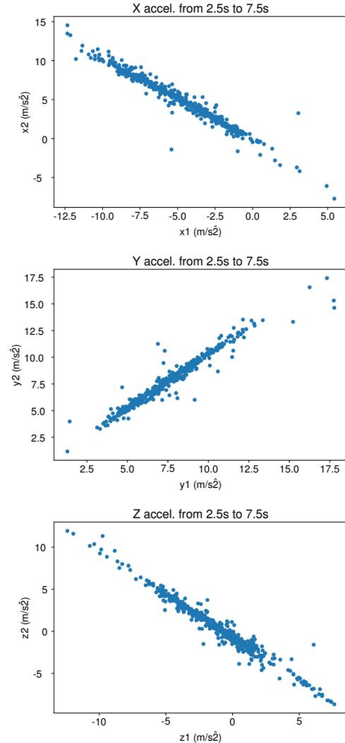
Fig. 3. Graphs of the acceleration of the Nexus 5X ( $x_1/y_1/z_1$ ) against the Nexus 5 ( $x_2/y_2/z_2$ ) while physically taped together over the same period of time.
