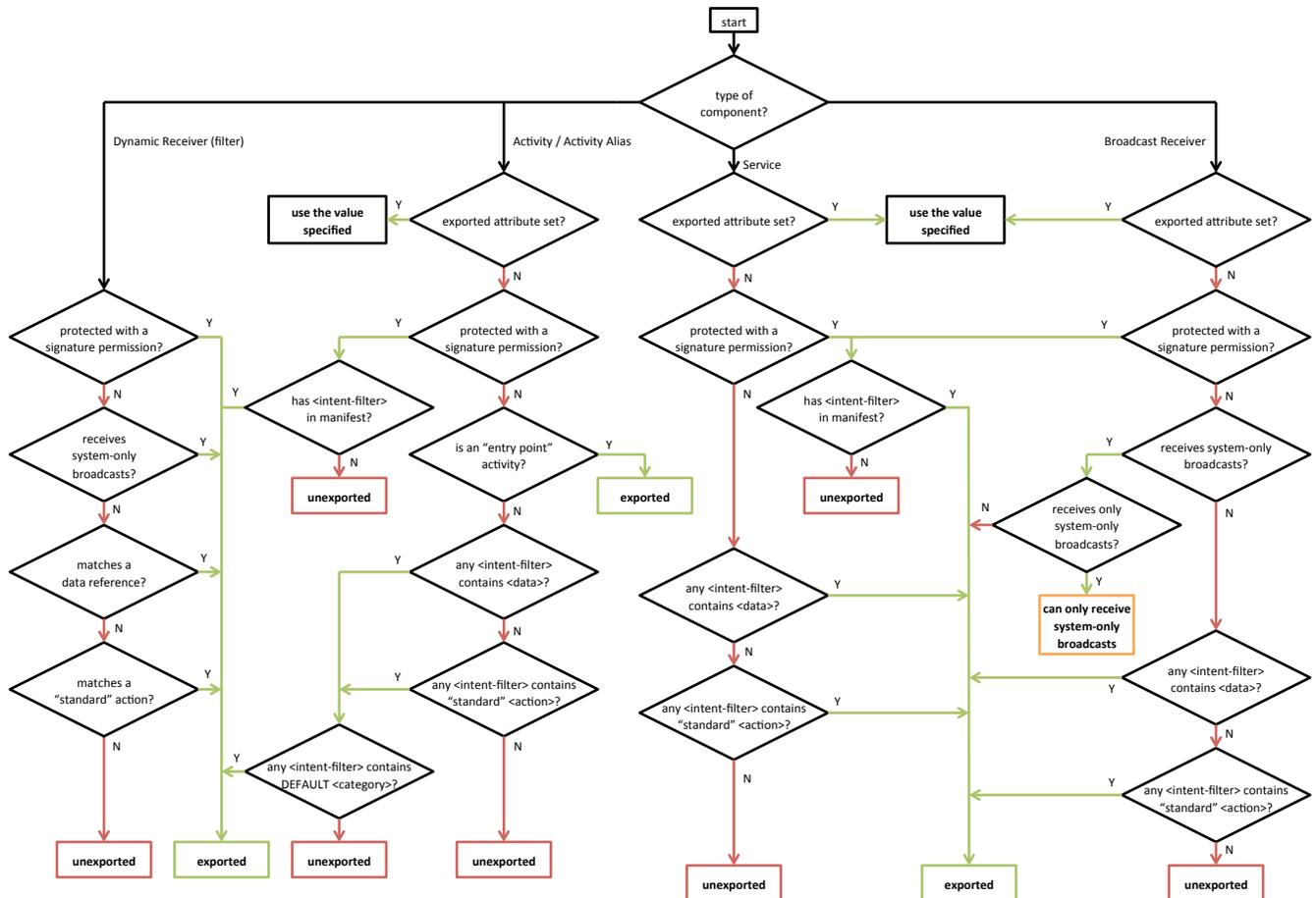
Figure 6: Our heuristic for when components should be exported.
