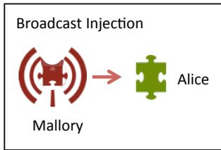
**Figure 4: Broadcast Injection: Mallory’s component broadcasts to Alice’s exported Broadcast Receiver. Alice thinks the broadcast comes from her own component.**
