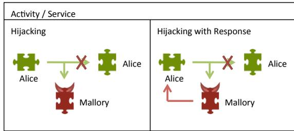
**Figure 3: Activity/Service Hijacking (left): Alice’s component unintentionally starts Mallory’s component instead of her own. False Response (right): Mallory’s component returns a malicious result to Alice’s component. Alice thinks the result comes from her own component.**
