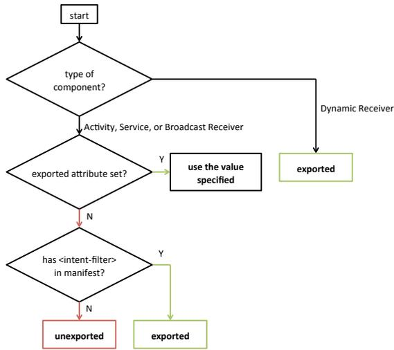
Figure 1: Android exports components that declare an Intent Filter or are explicitly marked for export. Dynamic Receivers are always public.
