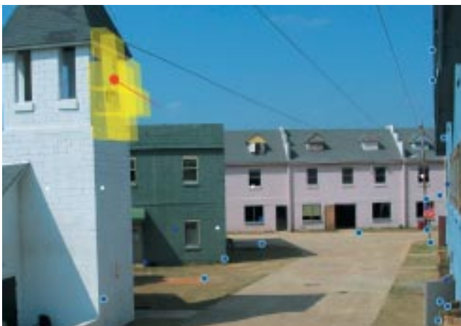
GUNSHOT LOCATION (red) was triangulated within seconds by a network of motes (blue dots) containing sound and shock-wave sensors.
