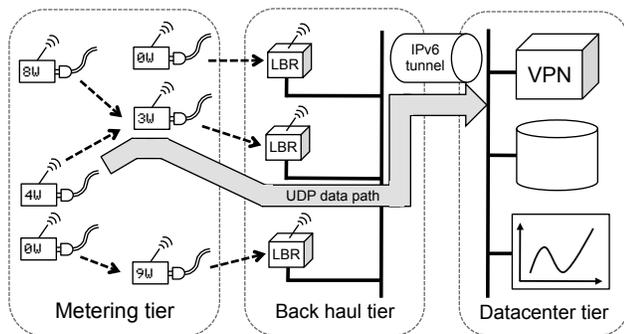
Figure 2: System design. The metering tier, left, forms an IPv6 mesh network of 802.15.4 links and transmits metering data through the backhaul tier comprised of load-balancing routers, center; these routers communicate with each other using the building’s Ethernet. The UDP data packets travel over an IPv6 tunnel from the building to the Internet where they reach the database, located in a datacenter.
