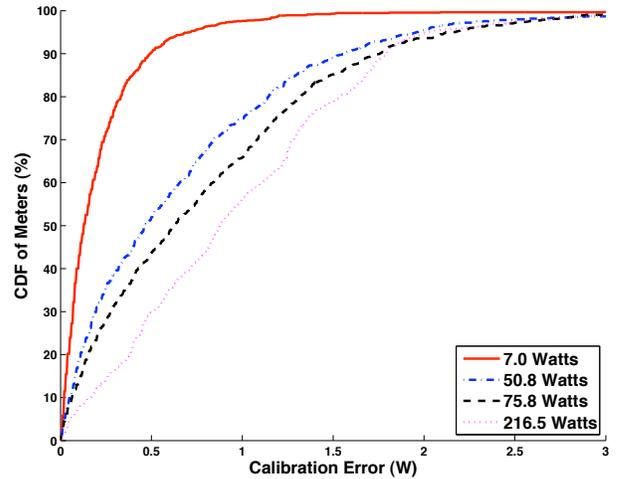
Figure 7: Error of calibrated meters at four load levels.
