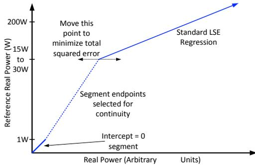
Figure 6: Selection of piecewise linear calibration coefficients.
