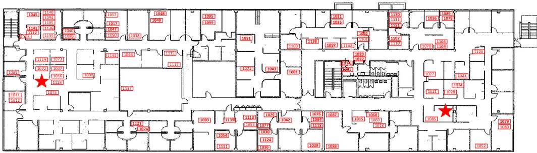
Figure 1: The third floor of the deployment. Small boxes are meters, while the two stars are LBRs.
