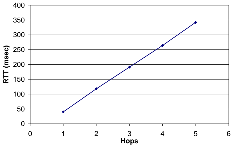
Figure 4. Round trip times for various route lengths. Note that one hop measures the time for a message between the Host PC and base station device.
