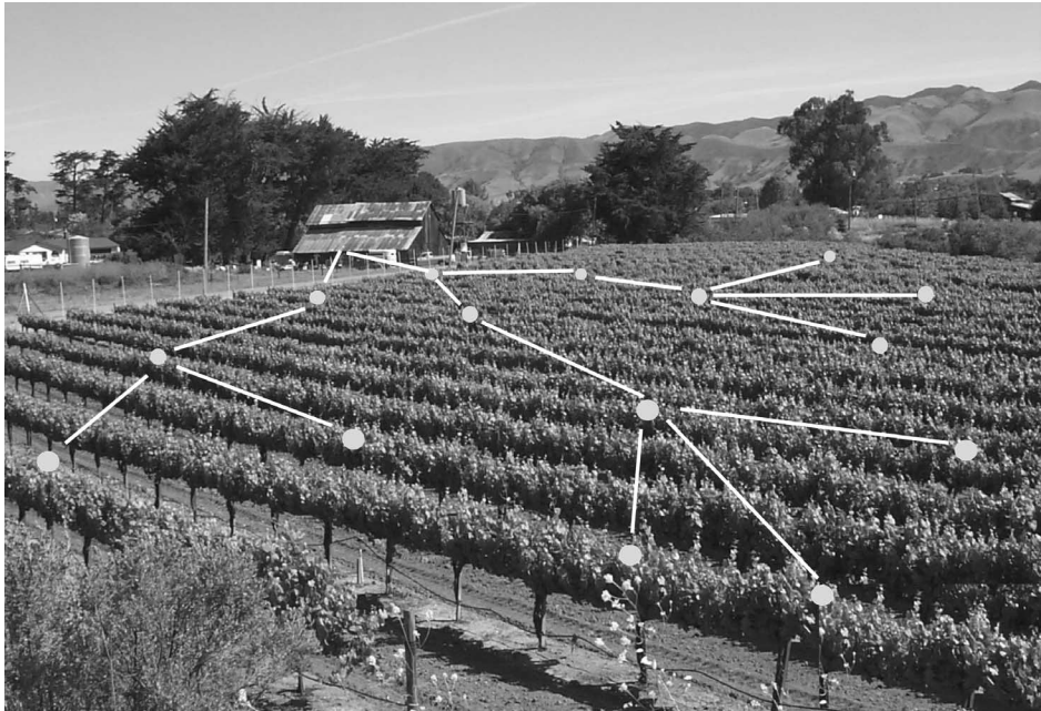
Figure 1. Ad hoc, wireless embedded network for precision agriculture. Sensors detect temperature, light levels, and soil moisture at hundreds of points across a field. The system communicates the data over a multihop network for analysis.
