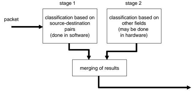
Fig. 7. Two stage classification architecture
