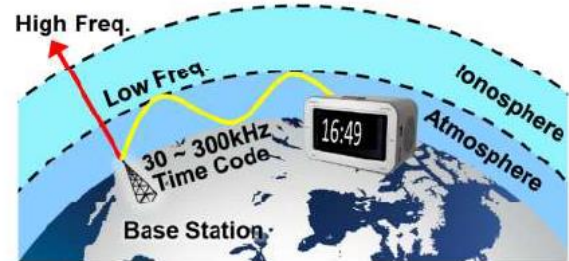
Figure 1: VLF and LF communication is possible over thousands of miles, practically crossing continents.
