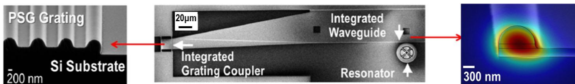
Fig. 5. SEMs of fabricated devices. (left) Cross-section of unreleased grating. (center) Wide-angle view of integrated waveguide and four-spoke optomechanical ring resonator. (right) FEM simulation of waveguide optical mode overlaid on SEM of half-ridge waveguide cross-section.
