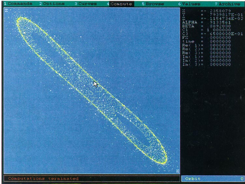
Fig. 4. Stable limit cycle (one trajectory in yellow for color picture) surrounding the three equilibria for \alpha = 0.9133561 , \beta = 0.88920 , and c_3 = -0.065 . The unstable limit cycles are not shown in the figure. (The limits of the axes are: x_{\min} = -0.5 , x_{\max} = 0.5 ; z_{\min} = -0.5 , z_{\max} = 0.5 .)
