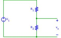
In this circuit,  $R_2$  represents the strain gauge and  $R_1$  is an auxilliary resistor with value  $R_o$ . Use  $V_1 = 3.3$  V unless otherwise indicated.
