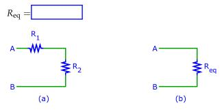
3. (D-4) Find the value of  $R_{eq}$  such that circuits (a) and (b) have the same I/V characteristic. Use  $R_1 = 9.8 \text{ k}\Omega$ ,  $R_2 = 4.9 \text{ k}\Omega$  and  $R_3 = 8.4 \text{ k}\Omega$ .
