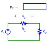
9. (F-7) Calculate the power  $P_{R_2}$  dissipated in resistor  $R_2$ . Parameter:  $V_1 = 13$  V,  $R_1 = 28$  k $\Omega$ ,  $R_2 = 24$  k $\Omega$ .
