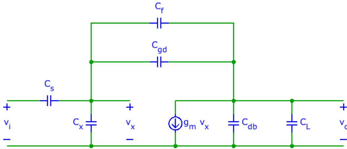
Absorb  $C_{gd}$ ,  $C_{db}$ , etc. in  $C_f$ ,  $C_L$ , ...
