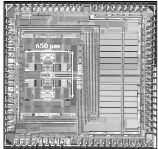
Fig. 6. Photomicrograph of the receiver.
