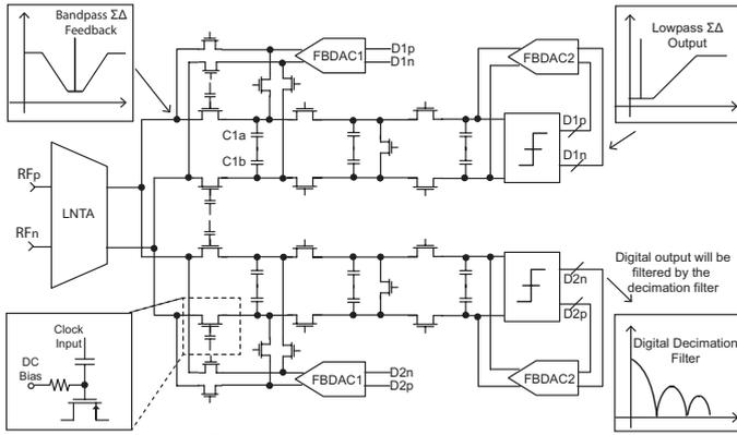
Fig. 2. Simplified schematic of the I-channel.
