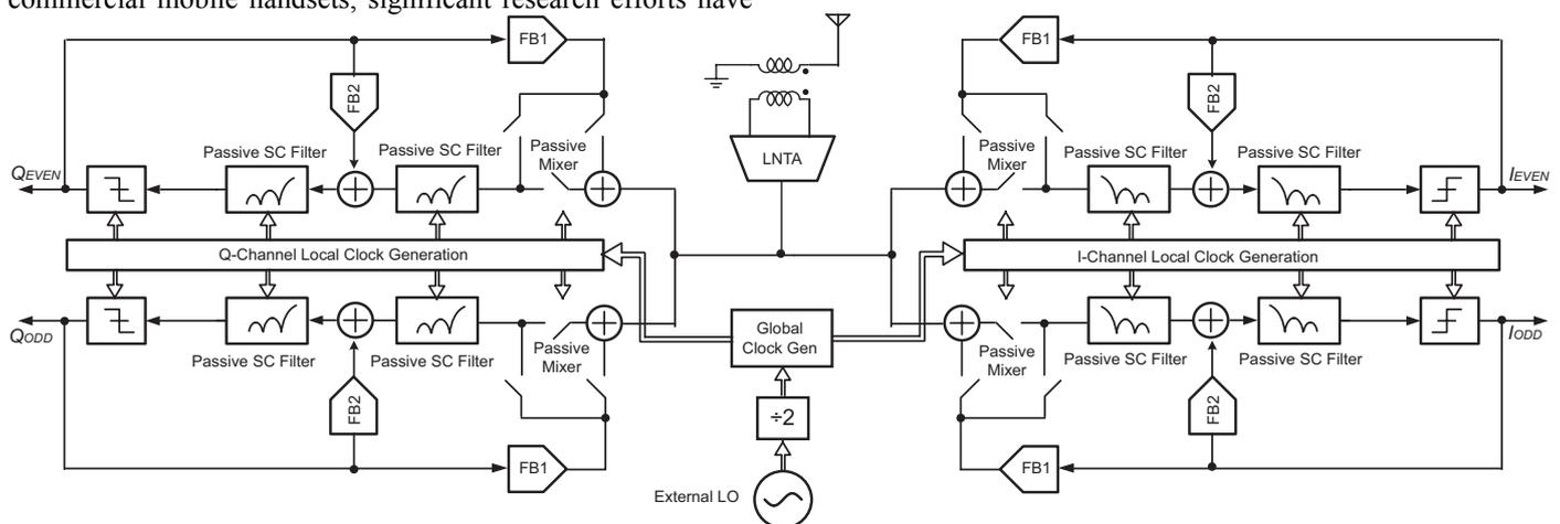
Fig. 1. Simplified block diagram of the receiver.
