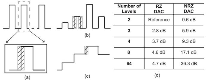
Fig. 3. Effect of clock jitter on RZ and NRZ DAC: a) illustration of the variation of clock pulse duration, b) RZ, c) NRZ, d) SNR improvement.
