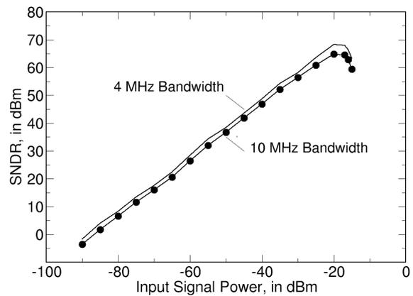
Fig. 7. Measured SNDR at  $2\text{ GHz}$  carrier frequency.
