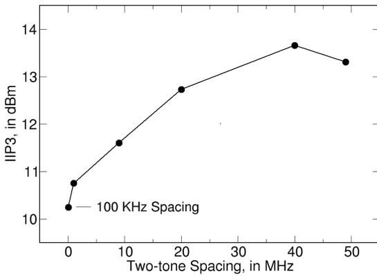
Fig. 10. IIP3 versus two-tone spacings at 2 GHz.
