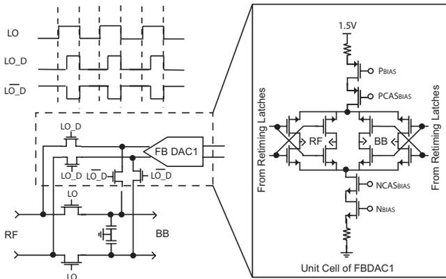
Fig. 5. Simplified schematic and clocking scheme for FBDAC1.
