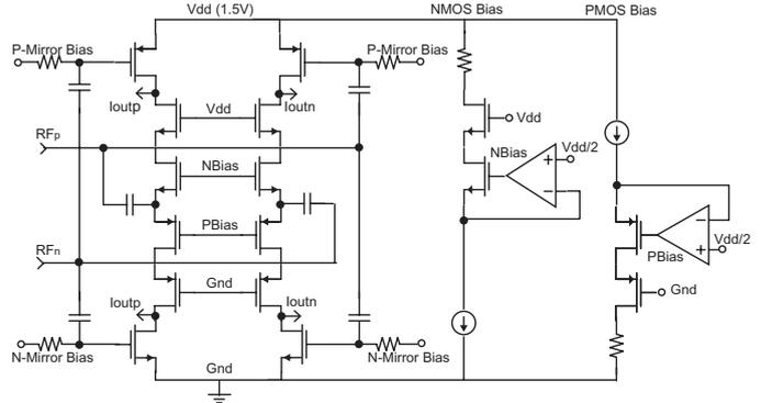
Fig. 4. Low-noise transconductance front-end with biasing.
