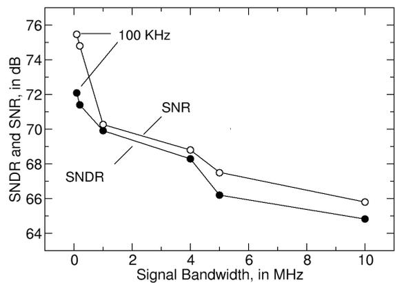
Fig. 8. Measured SNR and SNDR at  $2\text{ GHz}$  carrier frequency.
