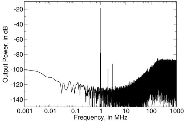
Fig. 9. Output spectrum at 2 GHz center frequency with input signal 1 MHz offset from the carrier.
