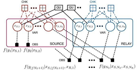
Fig. 3. Factor Graph: Systematic code at relay and scalar quantizer.
