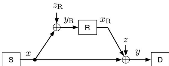
Fig. 1. Half-Duplex Gaussian Relay Channel
