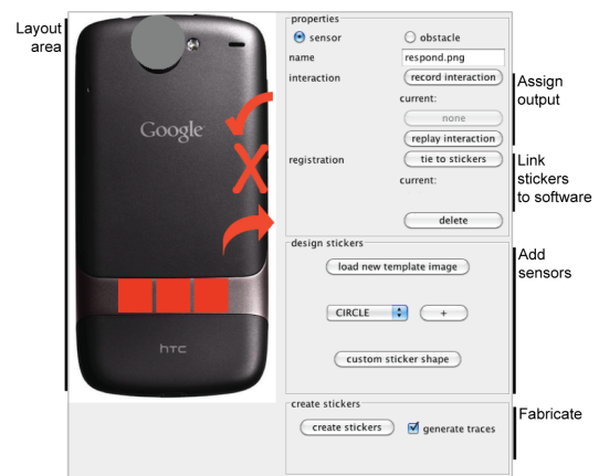
Figure 3: Midas’s sensor editor takes its cues from GUI editors: designers first lay out sensing areas through direct manipulation; they later define interactions for each sensor using a property inspector.
