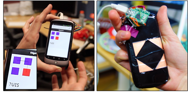
Figure 11: We implemented Wobbrock’s Edgewise on the back of a cell phone using a 2x2 pad and WebSocket events sent to a web page.
