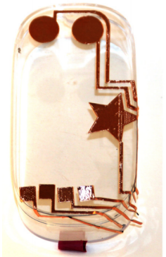
Figure 4: Midas is a tool for adding touch sensitive elements to any object. It uses a vinyl cutter to create conductive circuits for capacitive sensing.
