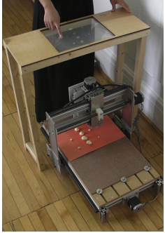
Figure 3: The Shaper is a tool for Interactive Fabrication. New fabrication machines can be designed with interaction in mind.
