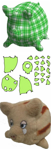
Figure 2: Plushie allows users to easily create plush toys through a sketch based interface. It uses a laser cutter to cut out fabric pieces, which the user assembles.
