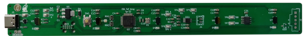
Figure 9: Example distance sensor array board. Port arrays enable the distance sensor array by exposing the shutdown pin for each individual device, while multipacking combines three discrete LEDs into an RGB LED.
