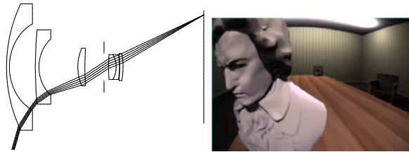
Fig. 5. Full lens simulations can exhibit aberrations that are not possible with thick lens simulations, such as appear in this image taken with a 16mm fish-eye lens. The image shows the lens' signature barrel distortion. (Courtesy of Craig E. Kolb [10] © 1995 ACM, Inc. Reprinted by permission.)
