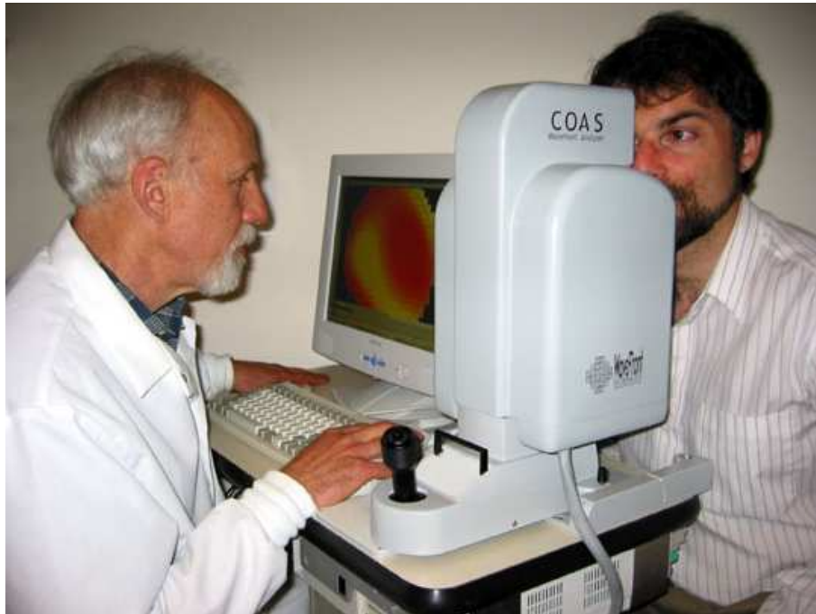
Fig. 3. Measuring the specific vision characteristics of a subject using a Shack-Hartmann wavefront aberrometry device.
