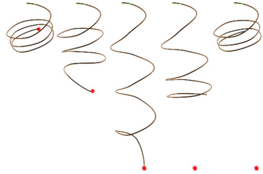
Fig. 8. Elongation of spring with 16 control points, E = 1.5e7 Pa, D = 1 cm.
