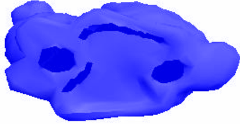
(a) Four holes in the mesh model
