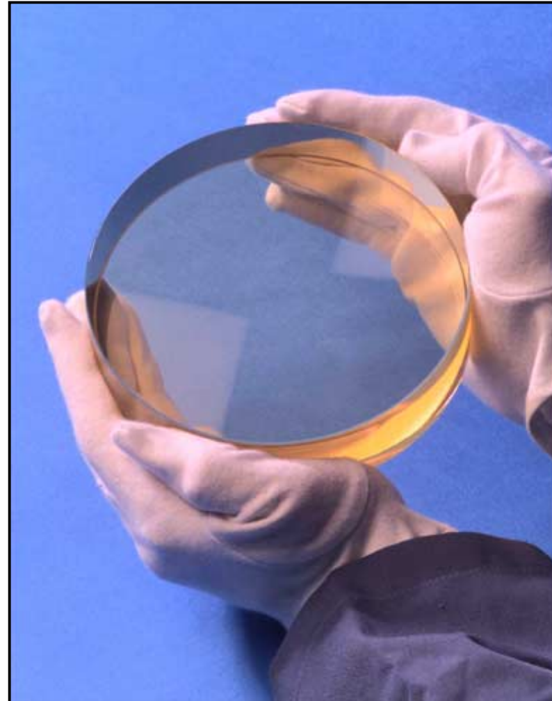
Tinsley Sample C Zerodur-M 150 mm diameter
