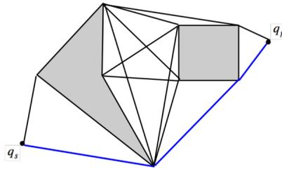
*A path is found from  $q_s$  to  $q_g$  by connecting mutually visible polygonal vertices and running graph search*
