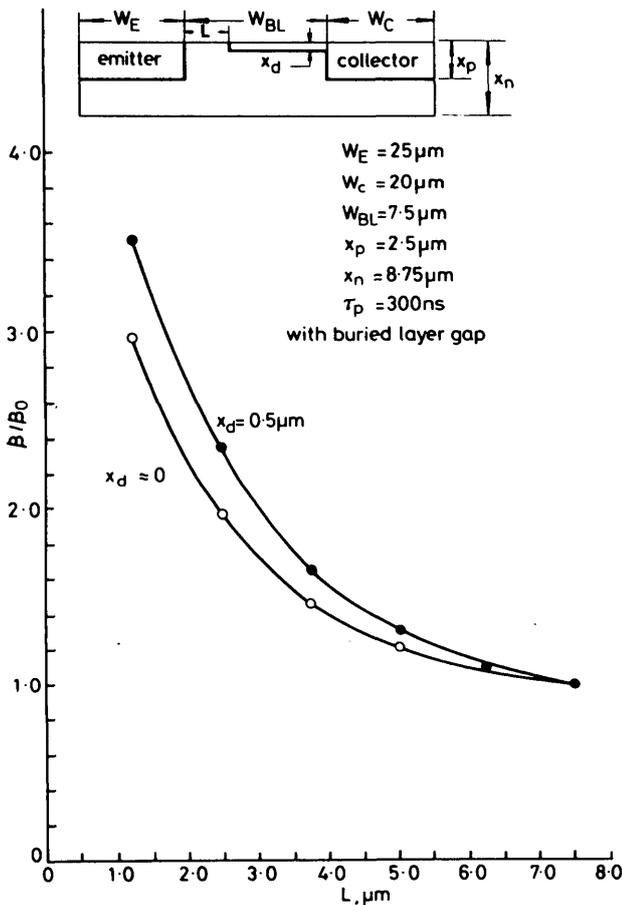
Fig. 5 Normalised current gain of lateral p-n-p transistor as a function of the spacing  $L$  between the emitter edge and the field plate for two values of the depletion layer width  $X_d$
