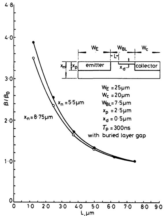
Fig. 6 Normalised current gain of lateral p-n-p transistor as a function of the spacing  $L$  between the emitter edge and field plate for two values of epilayer thickness  $X_n$
