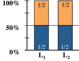
**Figure 4:** Bandwidth consumptions of tenant-*A* (orange) and tenant-*B* (dark blue) with correlation vectors  $\vec{d}_A = \langle \frac{1}{2}, 1 \rangle$  and  $\vec{d}_B = \langle 1, \frac{1}{6} \rangle$  using PS-P [45, 58, 59]. Both tenants run elastic-demand applications.
