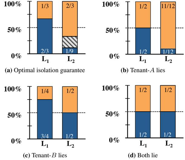
**Figure 5:** Bandwidth consumptions of tenant-*A* (orange) and tenant-*B* (dark blue) with correlation vectors  $\vec{d}_A = \langle \frac{1}{2}, 1 \rangle$  and  $\vec{d}_B = \langle 1, \frac{1}{6} \rangle$ , when both run elastic-demand applications. (a) Optimal isolation guarantee in the absence of work conservation. With work conservation, (b) tenant-*A* increases her progress at the expense of tenant-*B*, and (c) tenant-*B* can do the same, which results in (d) a prisoner’s dilemma.
