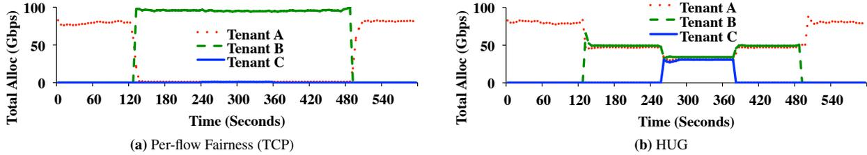
**Figure 10:** [EC2] Bandwidth consumptions of three tenants arriving over time in a 100-machine EC2 cluster. Each tenant has 100 VMs, but each uses a different communication pattern (§5.1.1). We observe that (a) using TCP, tenant-*B* dominates the network by creating more flows; (b) HUG isolates tenants *A* and *C* from tenant *B*.
