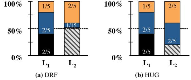
**Figure 14:** Hard tradeoff between work conservation and strategy-proofness. Adding one more tenant (tenant- $C$  in black) to Figure 5 with correlation vector  $\langle 1, 0 \rangle$  makes simultaneously achieving work conservation and optimal isolation guarantee impossible, even when all three have elastic demands.
