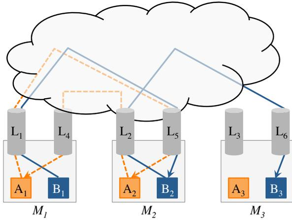
**Figure 3:** Two VMs from tenant-A (orange) and three from tenant-B (dark blue) and their communication patterns over a  $3 \times 3$  datacenter fabric. The network fabric has three uplinks ( $L_1$ - $L_3$ ) and three downlinks ( $L_4$ - $L_6$ ) corresponding to the three physical machines.
