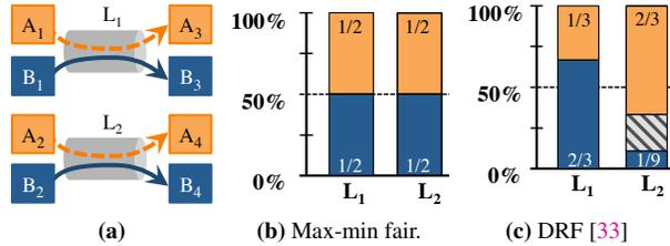
**Figure 1:** Bandwidth allocations in two independent links (a) for tenant-A (orange) with correlation vector  $\vec{d}_A = \langle \frac{1}{2}, 1 \rangle$  and tenant-B (dark blue) with  $\vec{d}_B = \langle 1, \frac{1}{6} \rangle$ . Shaded portions are not allocated to any tenant.
