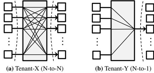
**Figure 9:** Communication patterns of tenant-X and tenant-Y with (a) two minimum cuts of size  $P$ , where  $P$  is the number of fabric ports, and (b) one minimum cut of size 1. The size of the minimum cut of a communication pattern determines its effective bandwidth even if it were placed alone.
