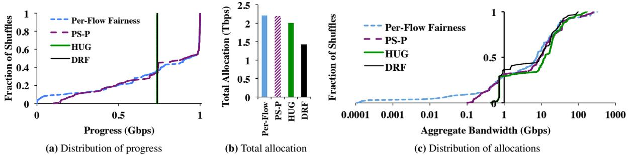
**Figure 11:** [Simulation] HUG ensures higher isolation guarantee than high-utilization schemes like per-flow fairness and PS-P, and provides higher utilization than multi-resource fairness schemes like DRF.
