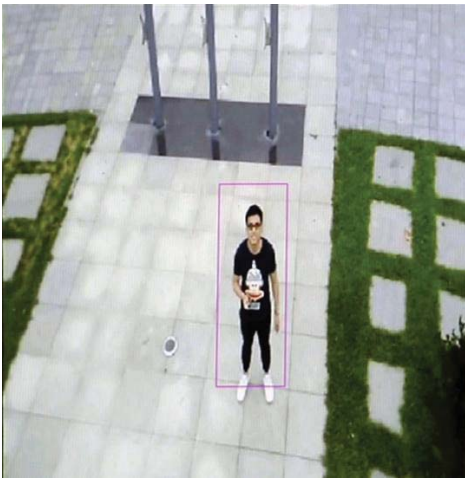
Fig. 14. Pedestrian detection result using YOLO. The purple box shows the detected target.
