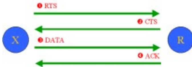
Figure 1: Signaling Between a Transmitter (X) and a Receiver (R) for Addressed Messages
