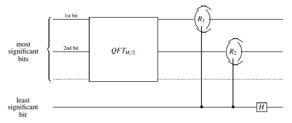
Figure 3: Circuit for quantum Fourier transform
