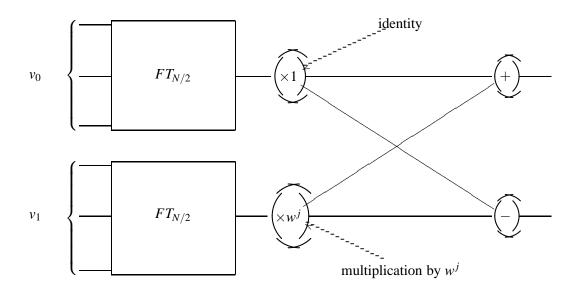
Figure 2: A circuit for classical fast Fourier transform
