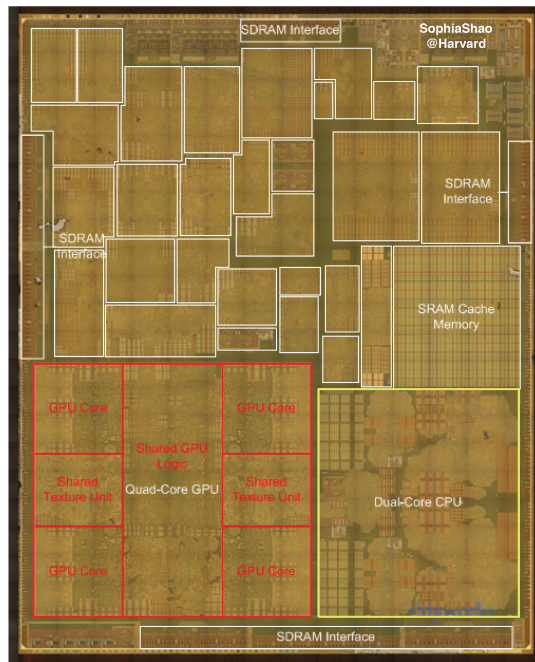
Figure 1.15: An annotated die photo of an Apple A8 (iPhone 6) SoC. The yellow box on the lower right is a dual-core CPU, and the red box on the lower left is a quad-core GPU. More than half of the die area is dedicated to non-CPU, non-GPU blocks (white boxes), most of which are application-specific accelerators. The original die photo is from Chipworks 4 .
