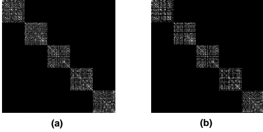
Fig. 5. Two examples of the matrix U^*(U^*)^T computed from the data corrupted by sample-specific corruptions. (a) The magnitudes of the corruptions are set to be about 0.7 times as large as the samples. Considering |U^*(U^*)^T| as an affinity matrix, the average affinity degree of the corrupted samples is about 40, which means that the corrupted samples can be projected back onto their respective subspaces. (b) The magnitudes of the corruptions are set to be about 3.5 times as large as the samples. The affinity degrees of the corrupted samples are all zero, which means that the corrupted samples are treated as outliers. In these experiments, the data samples are generated in the same way as in Fig.4. Then, 10% samples are randomly chosen to be corrupted by additive errors of Gaussian distribution. For each experiment, the parameter \lambda is carefully determined such that the column supports of E^* identify the indices of the corrupted samples.
