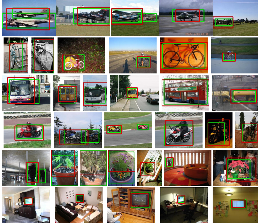
Figure 5: Red rectangles: object discovery results of ADMM on the challenging PASCAL 2007. Green rectangles: annotated object ground-truth. From top to bottom: aeroplane, bicycle, bus, motorbike, plotted-plants and tv-monitors.
