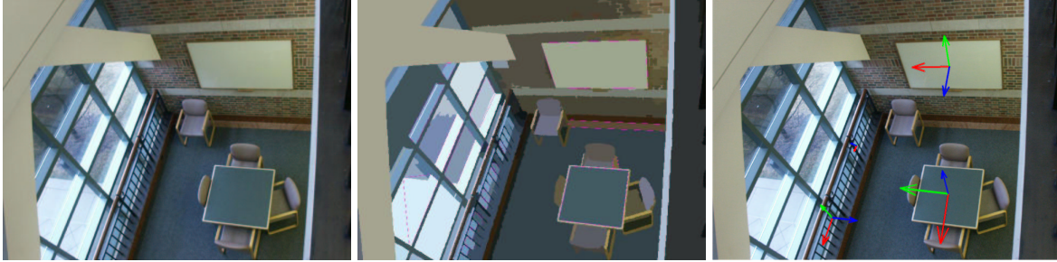
Figure 11: Left: original image. Middle: image segmentation and polygon fitting. Right: symmetry cells detected and extracted – an object frame (in RGB color) is attached to each symmetry cell.
