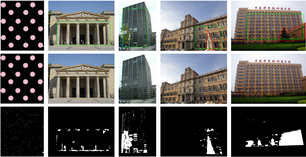
Fig. 10. Realistic repairing results. First row: input images where the green windows denote the input windows to our system, and red contours denote the initial error supports to our system. Second row: repairing images by our method. Third row: estimated final error supports by our method.
