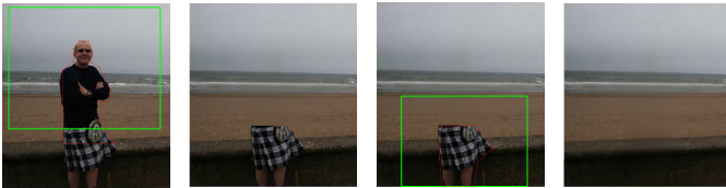
Fig. 13. Two regions with different distortion. The first image is the input image; the second image is the result after our method applied to the top-half; the third image is to apply our method to the bottom half; the last image is the final result.
