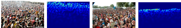
Figure 2: Original images and corresponding crowd density maps obtained by convolving geometry-adaptive Gaussian kernels.
