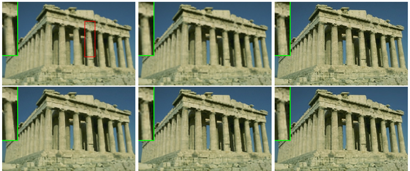
Fig. 5. Results on an image of the Parthenon with magnification factor 3 and corresponding RMSEs. Top row: low-resolution input, Bicubic interpolation (RMSE: 12.724), BP (RMSE: 12.131). Bottom row: NE (RMSE: 13.556), SE [7] (RMSE: 12.228), and our method (RMSE: 11.817 ).
