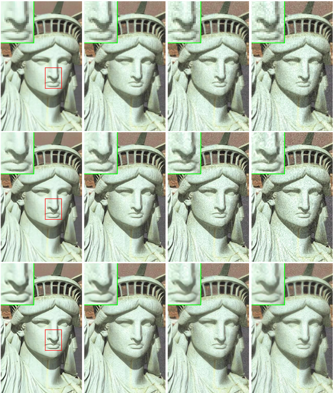
Fig. 12. Performance evaluation of our proposed algorithm on noisy data. Noise level (standard deviation of Gaussian noise) from left to right: 0, 4, 6 and 8. Top row: input images. Middle row: recovered images using NE [11] ( k = 13, 12, 9, 7 ). Bottom row: recovered images using our method ( \lambda = 0.1, 0.4, 0.6, 0.8 ).
