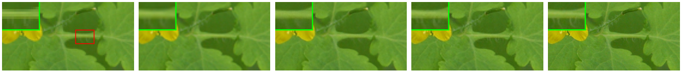
Fig. 3. Results of the flower image magnified by a factor of 3 and the corresponding RMSEs. Left to right: input, Bicubic interpolation (RMSE: 4.066), NE [11] (RMSE: 4.888), our method (RMSE: 3.761 ), and the original.
