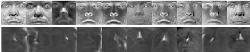
Fig. 7 Illustration of the first ten atoms of the illumination dictionary C . Top : Ad-Hoc Dictionary constructed from the first subject of YaleB database. Bottom : YaleB Dictionary learned from all the 38 subjects of YaleB.
