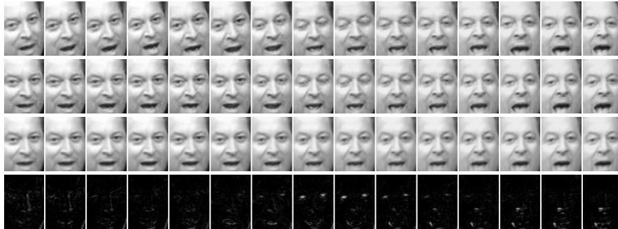
Fig. 12. Stabilization of faces in the video. 1st row: frames 1-15 from a 140-frame video, cropped by applying a face detector to each frame; 2nd row: input images after alignment D \circ \tau ; 3rd row: recovered low rank component A ; 4th row: sparse errors E .
